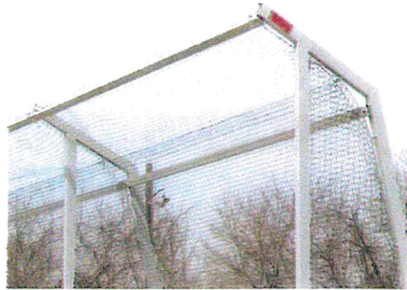
Canopy and Side-nets keep litter from escaping off the edges between adjacent units and over the top. Litter stays trapped even when the wind shifts and swirls.
