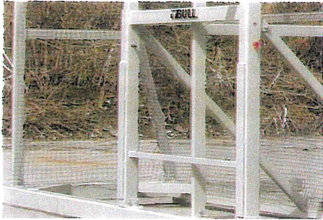
Wear Plates on Front Surfaces provide additional protection and stability. 3/4" thick steel plate welded on to bottom beam and hook supports provide this feature.
